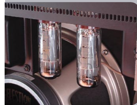
A pair of JJ Tesla E34L feeds the power amp section.
