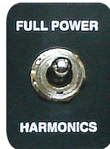
Penthode/triode mode for reduced output power of about 25W.
