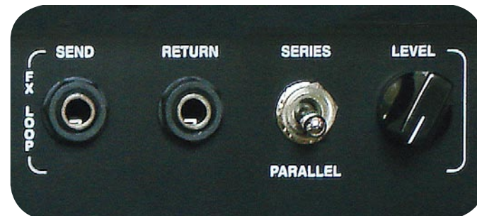
Series/parallel Fx loop. In parallel, the original sound of your amp is going unaltered to the cabinets and the effect quality is not affecting your tone.
